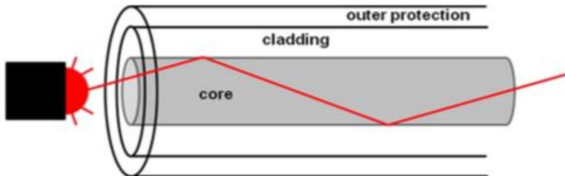
(Marking scheme: 1 mark for use of light; 1 mark for LED or laser; 1 mark for fibre core being glass; 1 mark for cladding; 2 marks for internal reflection)
