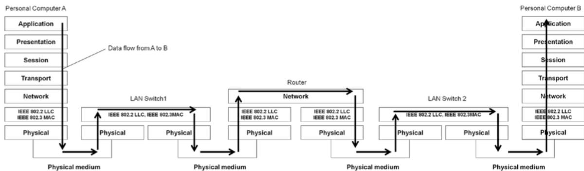
(Marking scheme: 2 marks for PC A showing all 7 layers; 2 marks for switch 1 showing layer 2 spanning both physical ports; 4 marks for the router showing layer 3 spanning both ports with each port having its own layers 1 and 2; 2 marks for LAN switch 2; and 2 marks for PC B. 2 marks for showing the data flow from PCA to PCB.)
