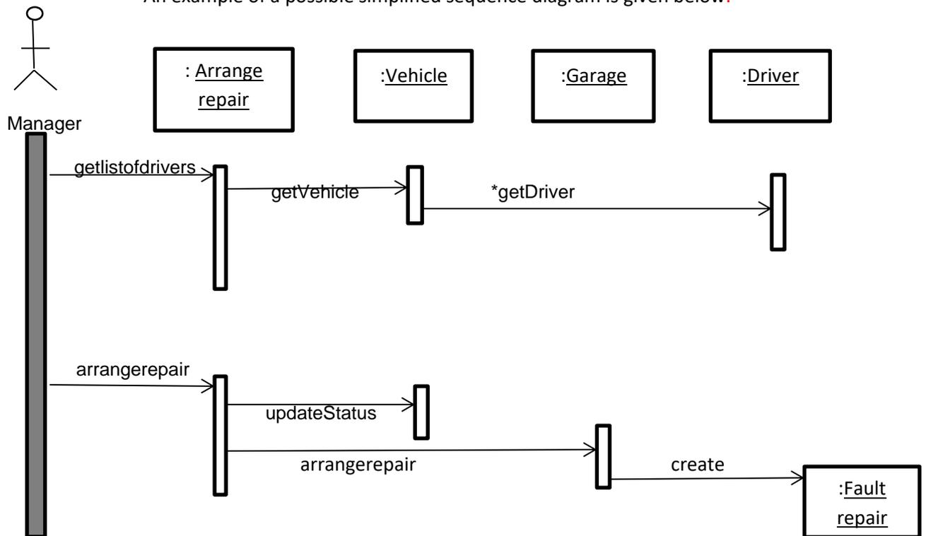
N.B.' Arrange repair' class represents both the boundary and control class for this use case.
